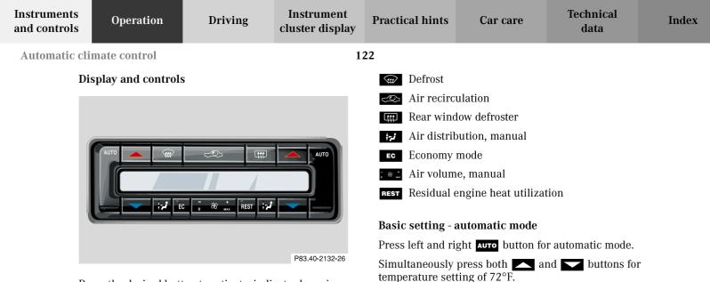
Press the desired button to activate, indicator lamp is on while activated.
